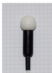
Calibrating Scalar PAR sensors (right) Sensor against 5 mm grid (left)
