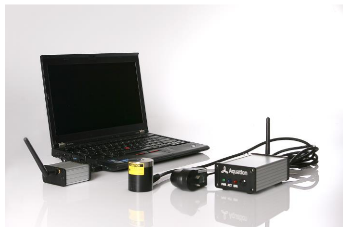
From left to right: USB Wireless unit, Fluorescence Sensor, Power plug, Wireless Interface box
