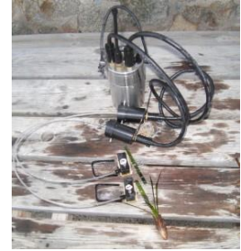
Above: Classic Fluorometer Standard 50m Fluorescence Sensor with light pipe extension, sample holder and Submersible Datalogger.
