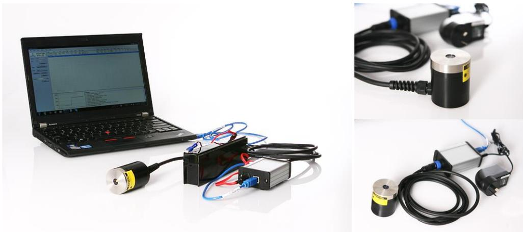
Aquation's **Classic Fluorometer USB Standard 3m** is designed for ease of handling, with the cable extending from the base of the sensor. The water resistant design enables convenient measurement of wet material including aquatic plants, algae and wet leaves. The small size of the fluorometer (1.8" diameter, 2.7" long), and its 12-24V capability makes it easy to use in the field.
